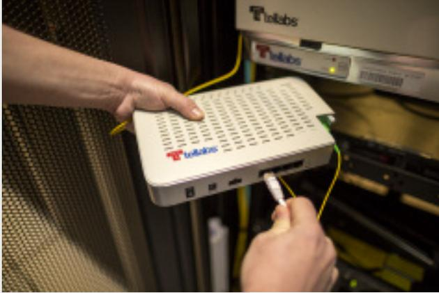
**Tellabs Optical network terminal** is usually installed on or under a user's desk to provide data and voice ports.
